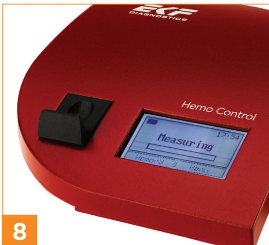
**8** The measurement will begin when the cuvette holder is closed.
