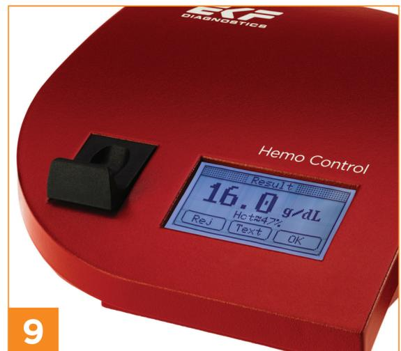
**9** The result is displayed on the screen after ca. 25 - 60 seconds. Press OK to leave the result screen.
