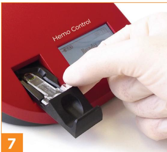
**7** Open the cuvette holder by pulling it out carefully. Insert the cuvette with the raised wing pointing to the right of the cuvette holder.
