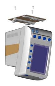
2 Lift the monitor and slide the link board into the groove of the top splint sideways. When the board goes halfway, pull down the pin on the back of the top splint to allow the board to go through. Keep pushing the board in until the pin rebounds and clicks into the hole. The edges of the Link board and the top splint should match perfectly at this moment.
