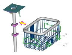
9 The lower basket and its concave are optional. First, install the concave block to a proper height of the stand post using two H screws. Then level the lower basket at the holes on the concave block and fix them with two H screws.
